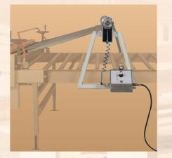
The optional roll stock feed attachment allows users to easily feed rolled stock laminate material (such as melamine, gator ply, fabric, etc). The unit is fitted with 3" (7.6 cm) core chucks and an air clutch which supplies consistent tension across the pay out bar.
