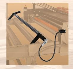
The optional hot knife adhesive cutter is a heated arm that reaches across the width of your laminator. The operator won't need to bend over the panel to cut adhesive. Instead, a quick flick of the wrist pushes the arm through the adhesive, making a fast and clean cut.
