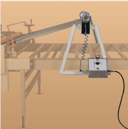
The optional roll stock feed attachment allows users to easily feed rolled stock laminate material (such as melamine, gator ply, fabric, etc). The unit is fitted with 3" (7.6 cm) core chucks and an air clutch which supplies consistent tension across the pay out bar.
